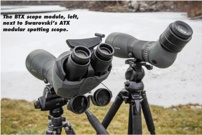
The BTX is a third option for the ocular component of these modular scopes, and combines the benefits and comfort of a binocular coupled with the power of a spotting scope.
